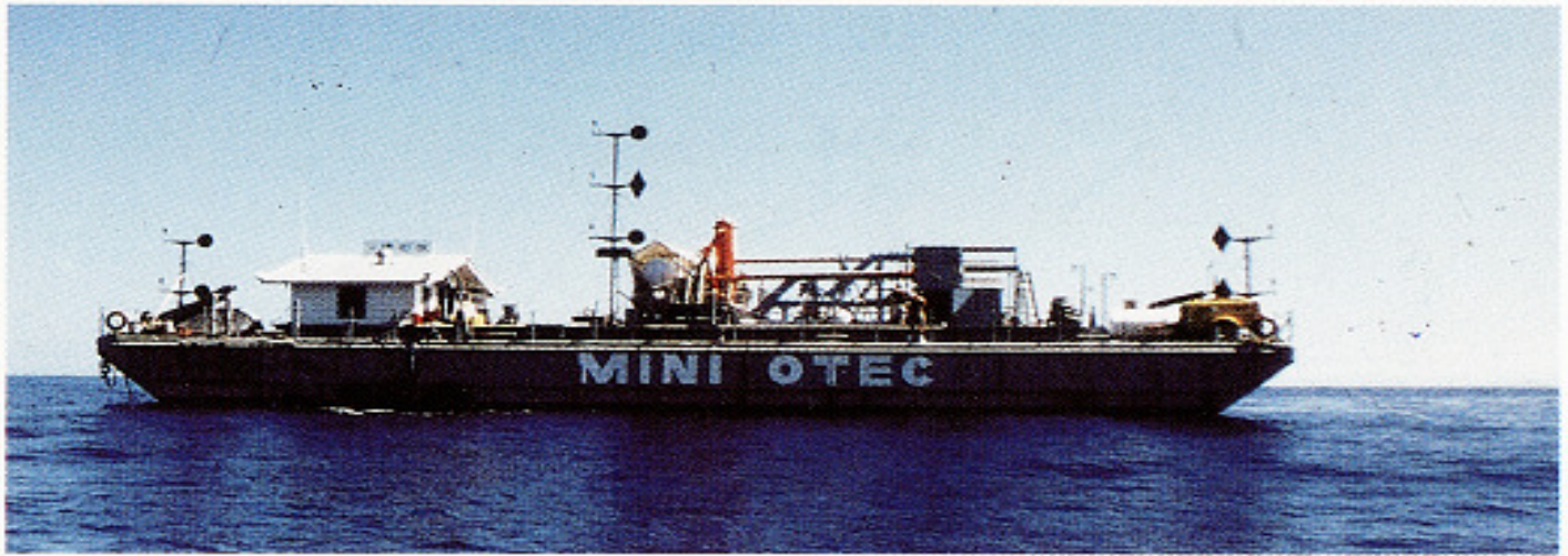
The first closed cycle Mini-OTEC plant to produce net power (15 kilowatts) at Keahole Point, Hawaii, in 1979
